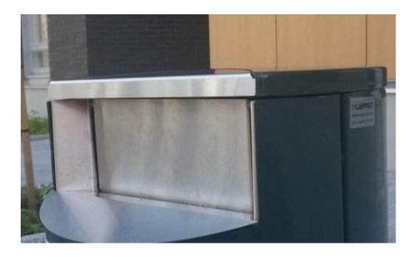
Bird stop is a stainless steel plate you can use to close the aperture to keep out birds, squirrels etc from the bin contents. When you push lightly the plate it opens inwards on it's upper hinges and you can drop litter into the bin. Product code for 60 and 100-liter CT-bins is CT-B60RST and for 30-liter bin CT-B30RST. You can insert the Bird stop plate also afterwards to a CT-bin, the fixing is simply two bolts in the upper corners.
