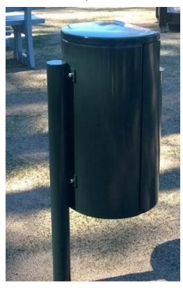
Post for deep mounting of 30 and 60 liter litter bins (CT and CL/Kita litter bins). Height 1200 mm, diameter 60 mm, material powder coated steel tube. Fits to the underground concrete clamp CT-C01 for deep mounting without wet concrete. The post has two fixed fastenings for litter bin so separate clamps are not needed and also bolts are included.
