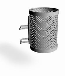
Litter bin for courtyards. Oskar is an open-top litter bin without a lid, and holds 35 litres. Oskar can either be set in the ground using poured foundations with the 40 mm post (NF2460), or affixed to the wall (NF2462) or an existing post measuring between 105 and 120 mm in diameter.
