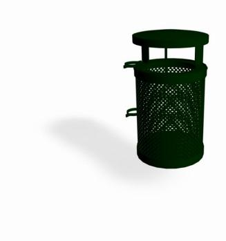
Litter-free playgrounds with Jakob. Jakob is a 35-litre litter bin. The litter bin has several fixing options - either set in poured foundations with a central post (50 mm) (NF2471), wall-mounted using a bracket for wall mounting (NF2472), or installed using a bracket on an existing post (105-120 mm). Jakob is made from 3 mm powder-coated steel.
