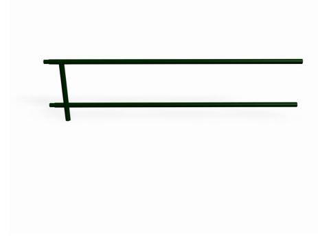
Extension section for railing NF7671A. Railing without seating plank; soft shapes in angled steel. With one mid-post 550 mm (c-c 2040 mm); designed for poured foundations. The images show the first sections.
