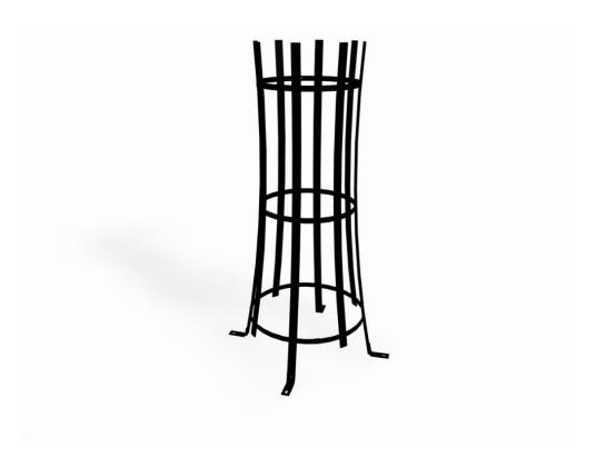
Decorative tree guard. This tree guard is an effective way of protecting trees in public environments. The tree guard posts are made from sheet steel; height from ground: 1600 mm, diameter 700 mm. For use together with ground grilles.
