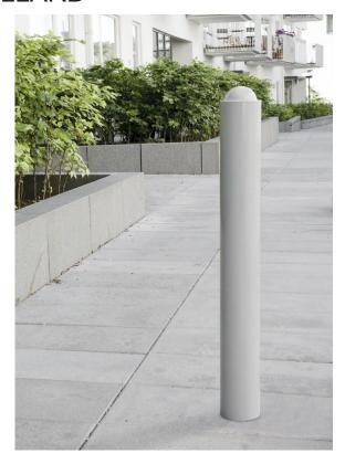
Removable bollard for roads and public squares. Cylindrical bollards for communal areas where pedestrians and drivers share the same space. Height 900 mm, c-c 180 mm. Designed for poured foundations. Can be removed from the base with a key.
