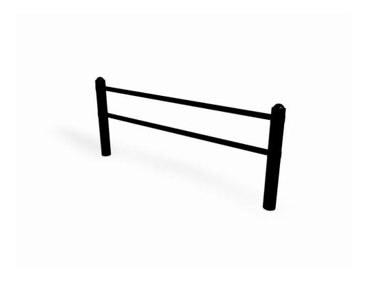
Flexible railing for public environments. Steel railing, 900 mm from the ground (c-c 2000 mm). The railing is affixed on the posts using a clamping ring and can therefore be angled as desired. Two bars in the middle.
