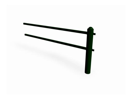
Extension section for railing NF9032. Single steel railing, 900 mm from the ground (c-c 2000 mm). The railing is affixed on the posts using a clamping ring and can therefore be angled as desired. Two bars in the middle.
