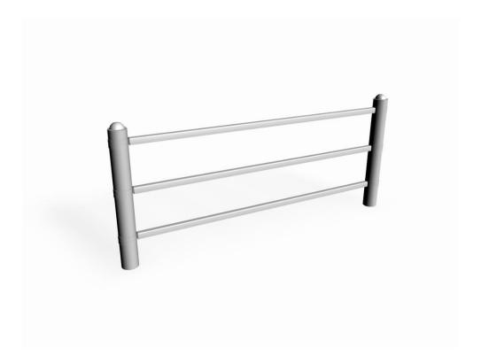
Flexible railing for public environments. Single steel railing, 900 mm from the ground (c-c 2000 mm). The railing is affixed on the posts using a clamping ring and can therefore be angled as desired. Three bars in the middle.
