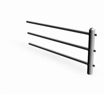
Extension section for railing NF9034. Single steel railing, 900 mm from the ground (c-c 2000 mm). The railing is affixed on the posts using a clamping ring and can therefore be angled as desired. Three bars in the middle.
