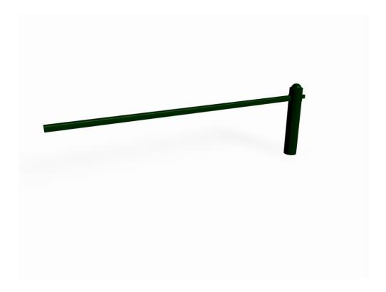
Edxtension section for railing NF9040. Single steel railing, 900 mm from the ground (c-c 2000 mm). The railing is affixed on the posts using a clamping ring and can therefore be angled as desired. One bar in the middle.
