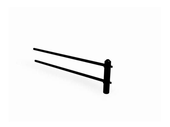
Extension section for railing NF9042. Single steel railing, 900 mm from the ground (c-c 2000 mm). The railing is affixed on the posts using a clamping ring and can therefore be angled as desired. Two bars in the middle.
