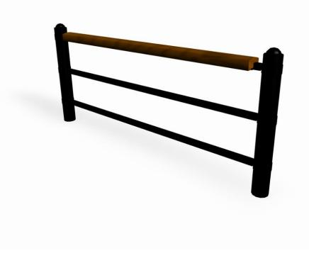
Flexible railing for train and bus stations. Steel railing with pine seating. With two mid-posts, height 900 mm. The seating lintel and mid-posts are affixed using a clamping ring on the posts, and can therefore be positioned at any angle.
