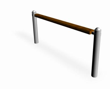
Flexible railing for train and bus stations. Steel railing with pine seating, height 900 mm. The seating lintel and mid-posts are affixed using a clamping ring on the posts, and can therefore be positioned at any angle.
