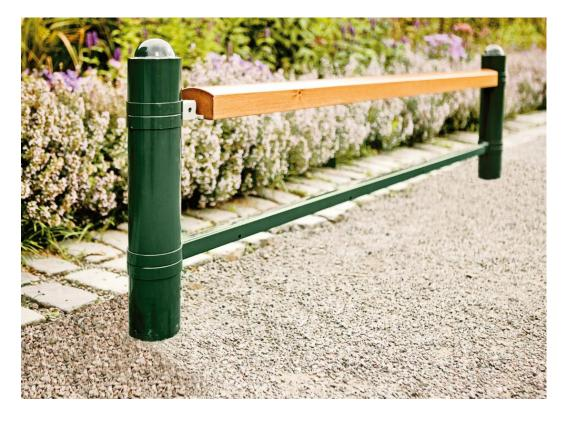
Flexible railing for train and bus stations. Steel railing with pine seating. With one mid-post, height 600 mm. The seating lintel and mid-posts are affixed using a clamping ring on the posts, and can therefore be positioned at any angle.
