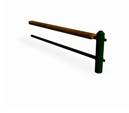
Extension section for railing NF9060. Steel railing with pine seating. With one mid-post, height 600 mm. The seating lintel and mid-posts are affixed using a clamping ring on the posts, and can therefore be positioned at any angle.
